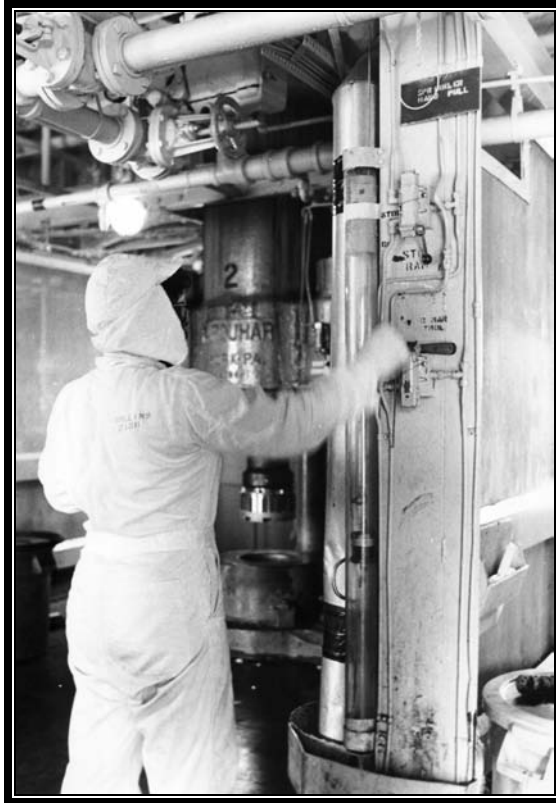
Plate 5.3 Operator using hydraulic blocking press, ca. 1965 (Photo courtesy US Army)
