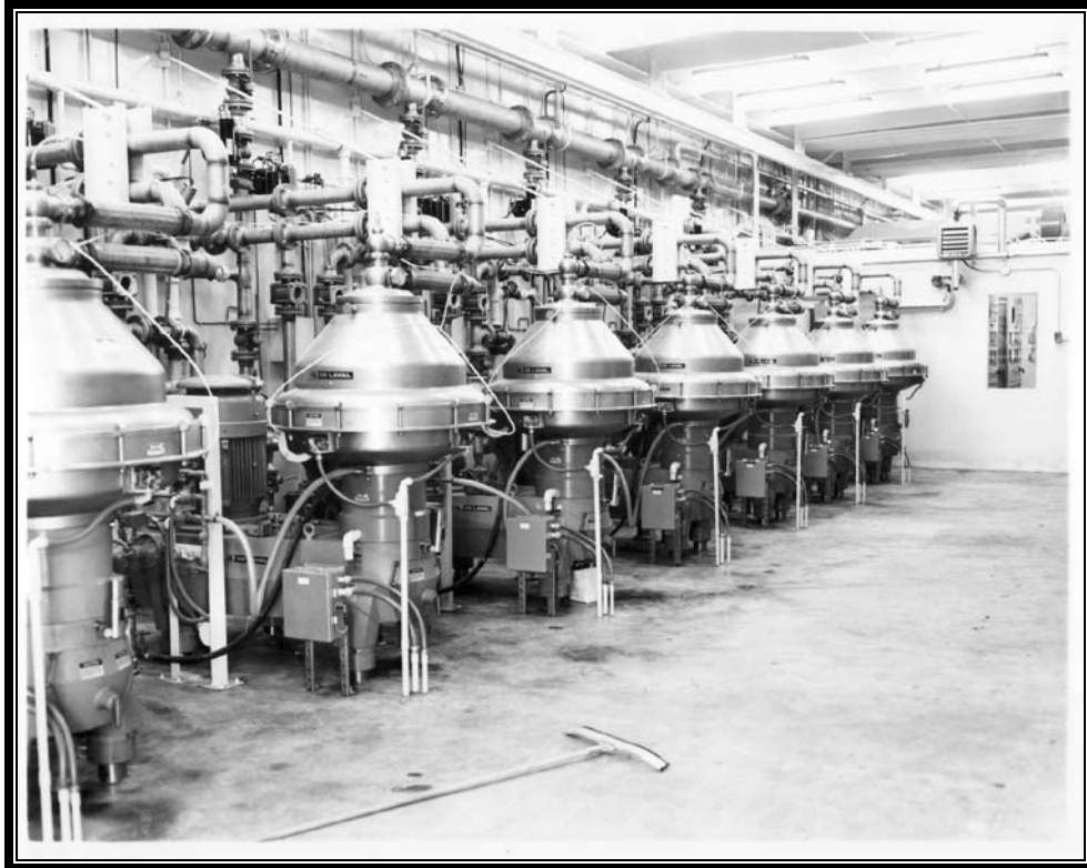
Plate 5.9 Centrifuges used in production of solventless propellants (Photo courtesy US Army)
