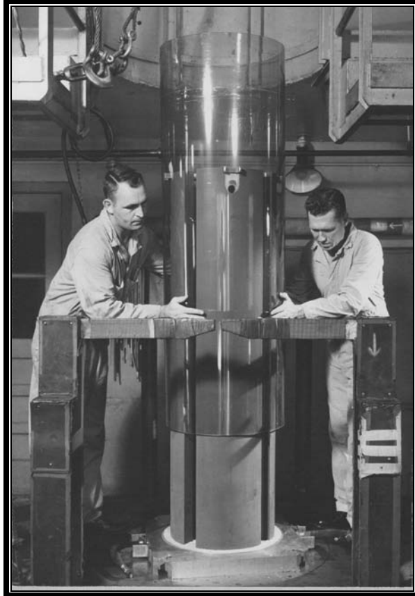
Plate 5.19 Preparing beaker for casting large rocket propellant grain (Photo courtesy US Army)
