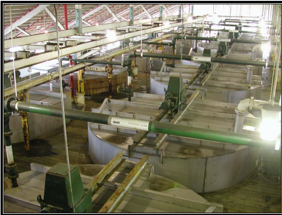
Plate 5.40 Mixing area for nitrocellulose, note that one wooden tank from the World War II era is still in use (Photo courtesy US Army)
