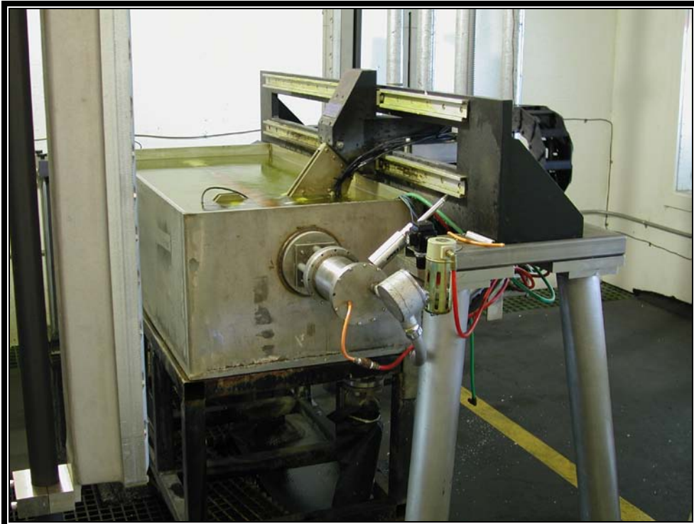
Plate 5.16 Inspection equipment for large propellant grains (Photo courtesy US Army)
