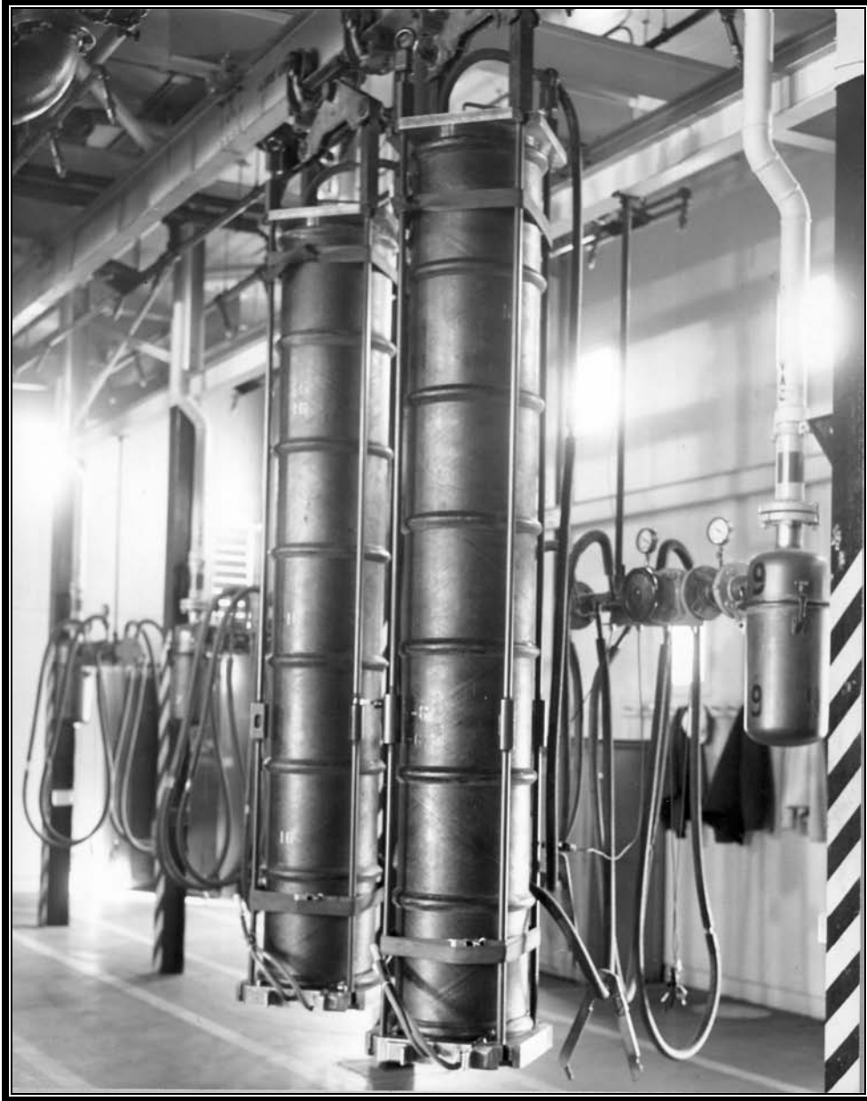
Plate 5.22 Curing area for rocket propellant grains, these are for HONEST JOHN missiles (Photo courtesy US Army)
