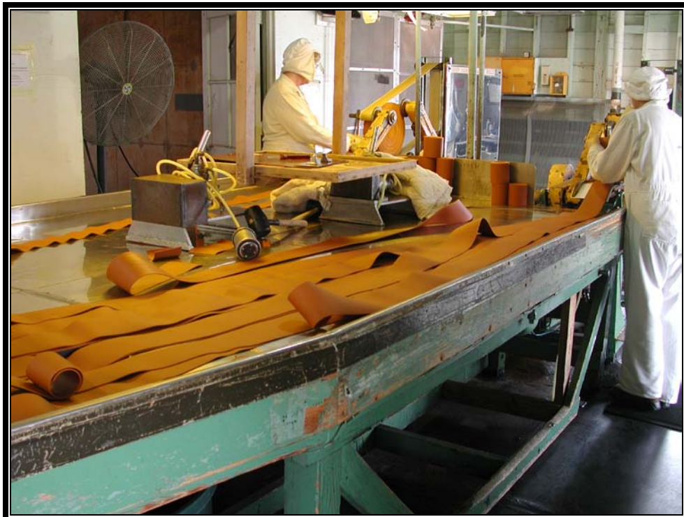
Plate 5.12 Strips of propellant at carpet roll machine (Photo courtesy US Army)
