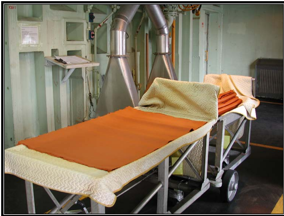
Plate 5.10 Sheets of solventless propellant (Photo courtesy US Army)
