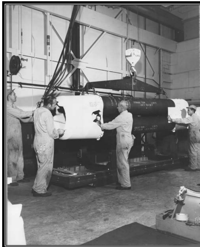
Plate 5.26 Preparing NIKE cluster of missile motors for shipment (Photo courtesy US Army)
