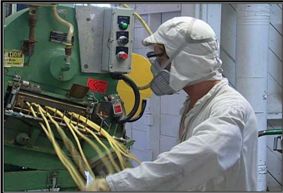
Plate 5.14 Extruding and cutting solventless propellant (Photo courtesy US Army)
