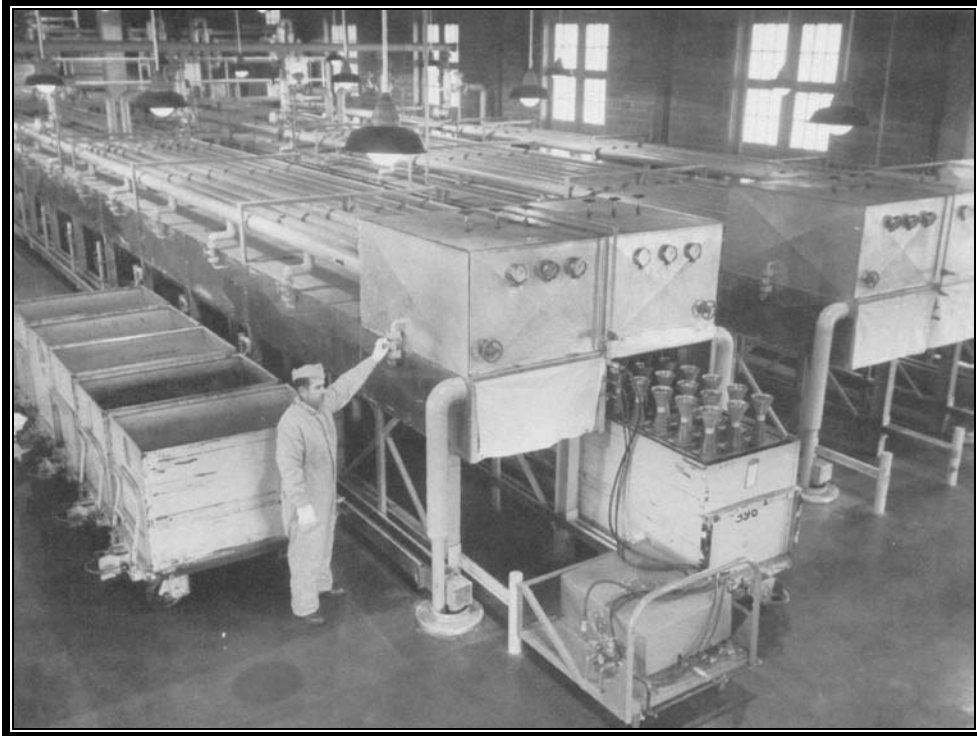
Plate 5.33. Conditioning ovens of SPCC process, ca. 1956 (Mason & Hanger Records, Eastern Kentucky University Archives, Richmond, KY)
