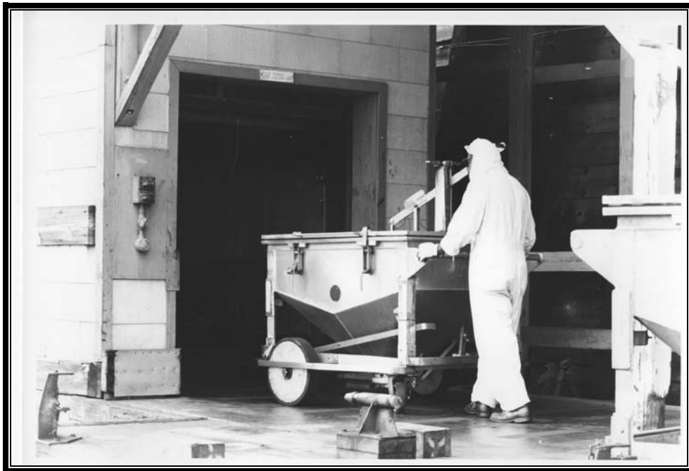
Plate 5.38 Buggy used for moving completed grains through the plant is loaded on the elevator of an air dry house (Photo courtesy US Army)
