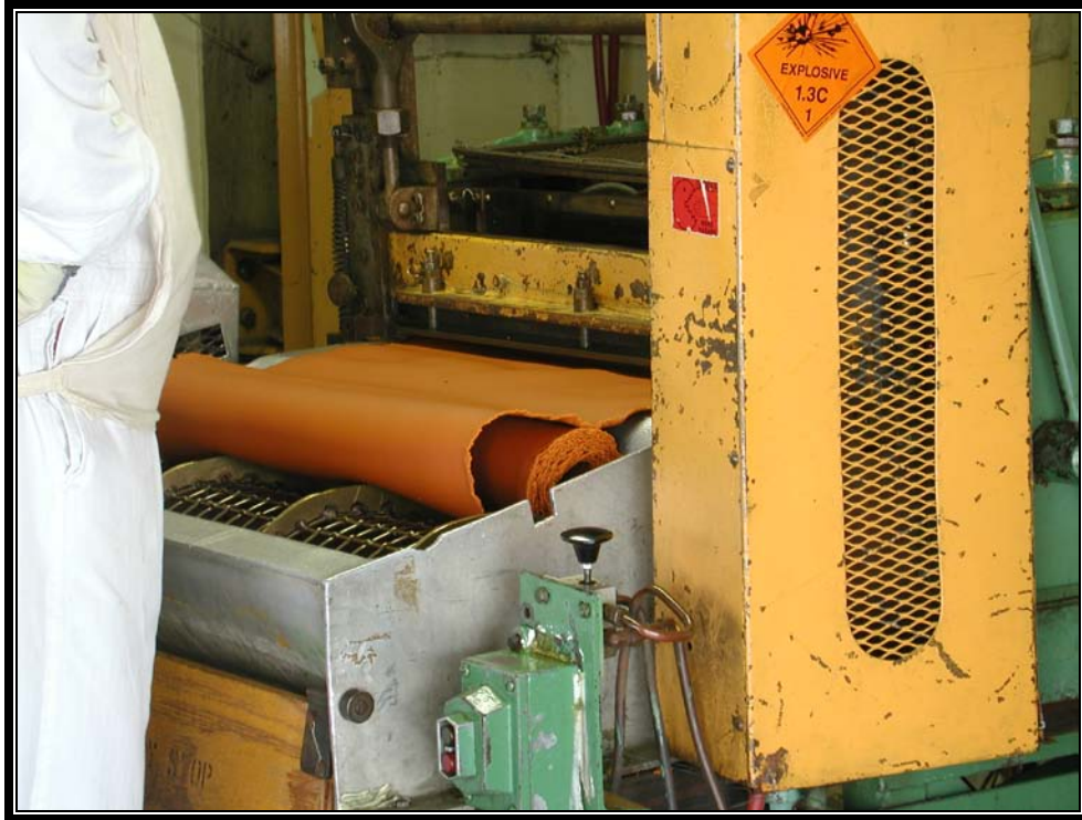
Plate 5.11 Machine used to cut sheets of propellant into strips (Photo courtesy US Army)
