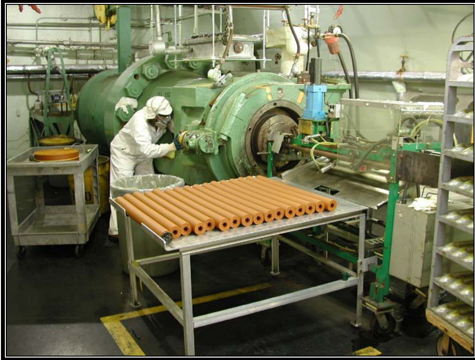
Plate 5.15 Extruding large rocket propellant grains (Photo courtesy US Army)
