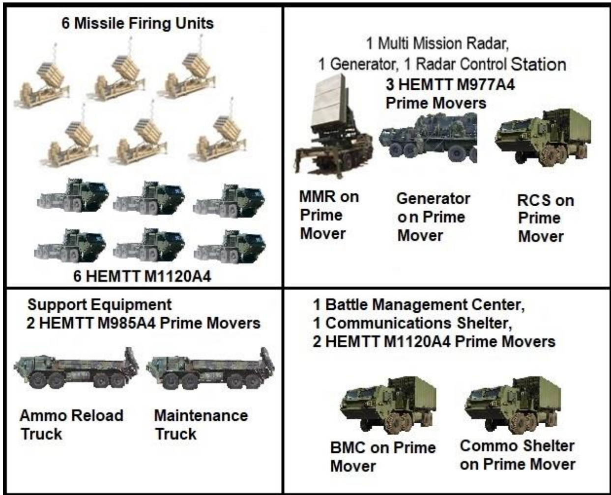
Figure 1.3-1 IDDS-A New Equipment and Transport Vehicles per Battery
