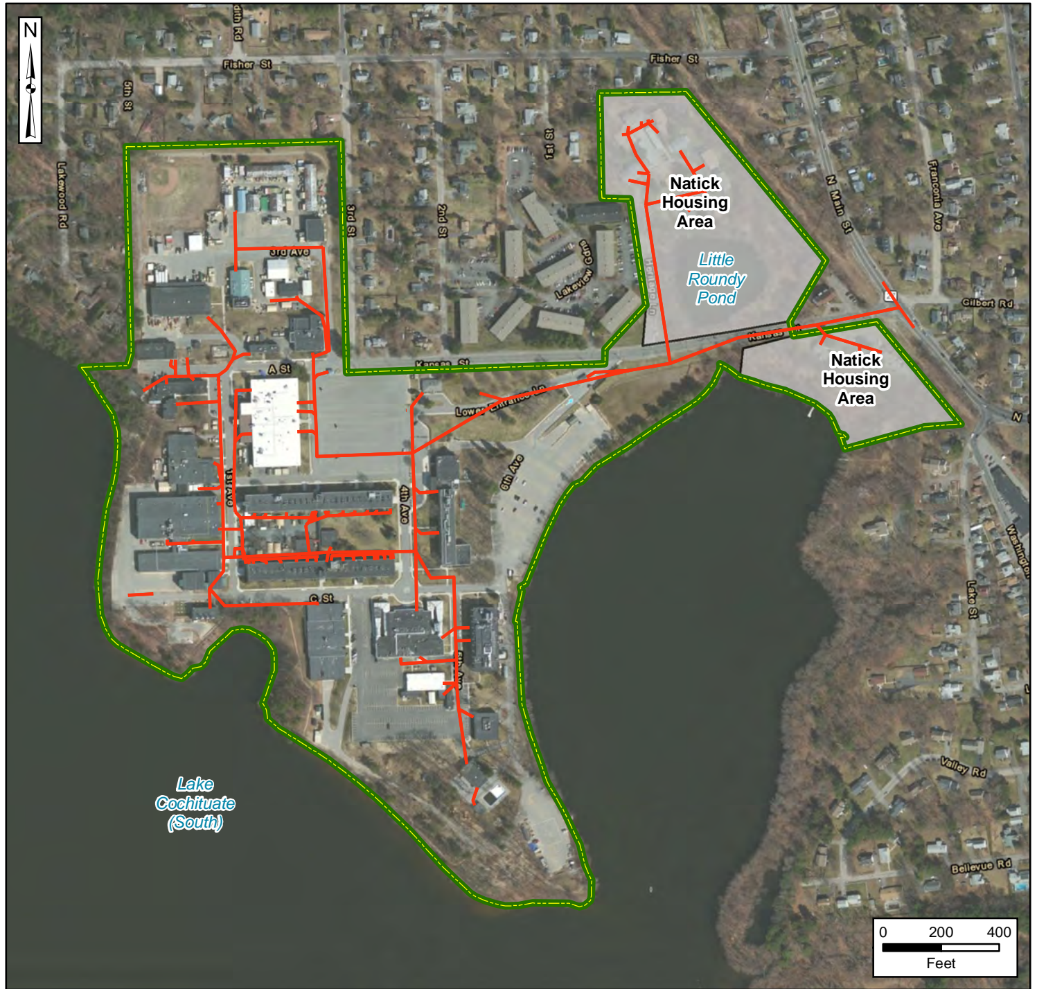
Figure 4-2 Sewer System Map
