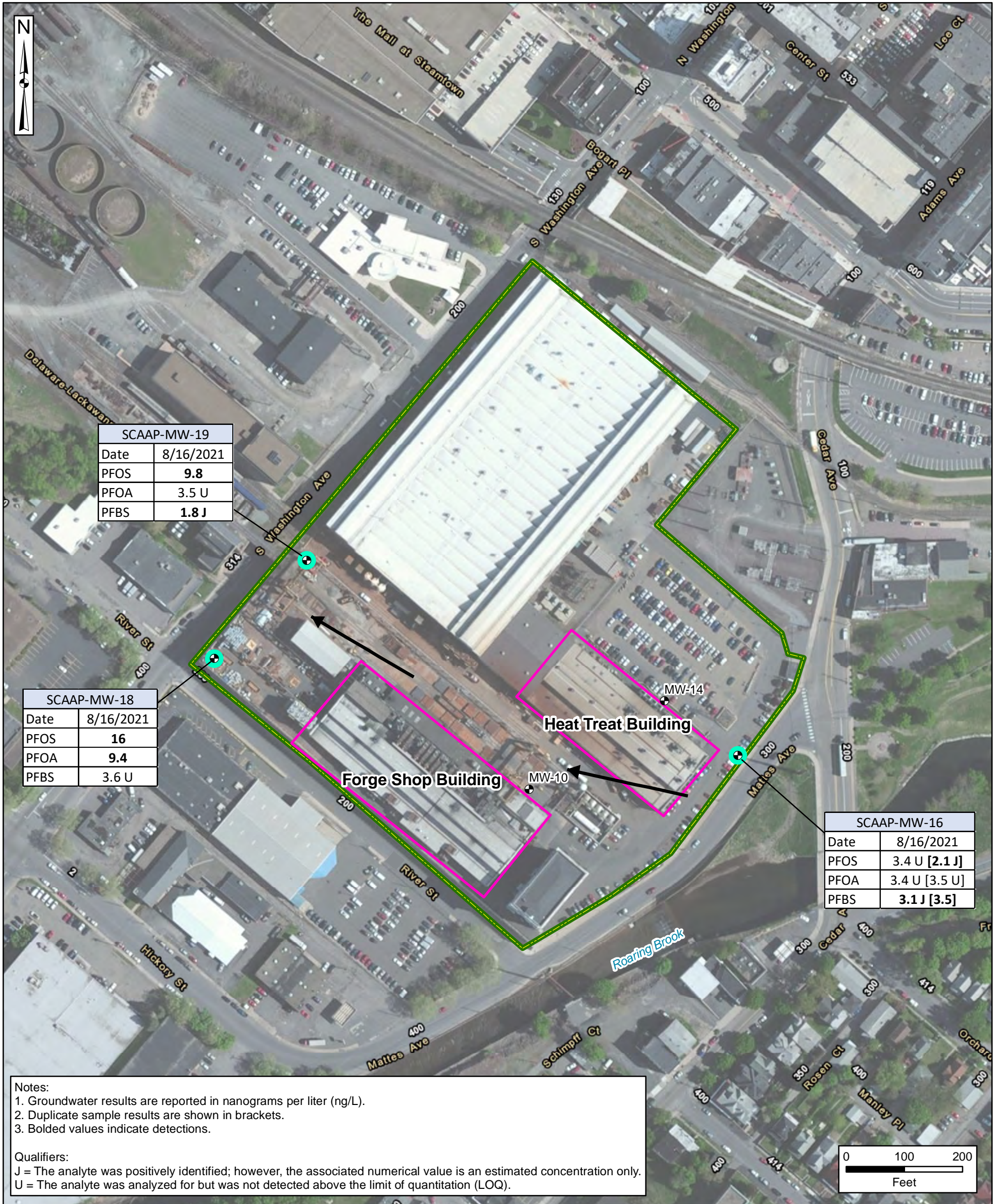
Figure 7-1 Forge Shop Building and Heat Treat Building AOPIs PFOS, PFOA, and PFBS Analytical Results
